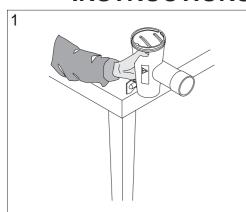
Place the housing on the edge of a table, the opening upwards, when the meat mincer is to be assembled.
