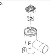
Knife and disc are placed on the shaft of the feed screw in the mentioned order.
