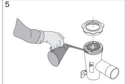
The thread of the housing shall be lubricated with grease before mounting of the ring. Use e.g. paraffin oil or castor oil, never salad oil.
