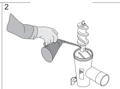
The shaft of the feed screw should be lubricated with grease before the feed screw is inserted into the housing. Use e.g. paraffin oil or castor oil, never salad oil
