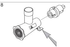
Mount the intermediate bearing on the meat mincer. The intermediate bearing must be pressed entirely into the meat mincer before tightening the thumb screw.
