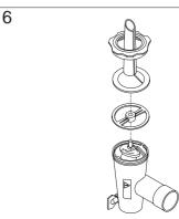
If a sausage tube is used, the distance ring of the sausage tube must be mounted on the shaft of the feed screw before the sausage tube and ring are mounted.
