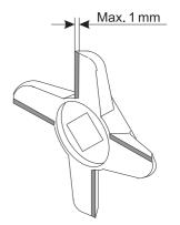
The knife must be replaced or grinded when the wearing surface on the side of the knife is more than **1 mm**. If this is not done, the mixer can be damaged, as the friction in the meat mincer is increased when the knife is worn.
